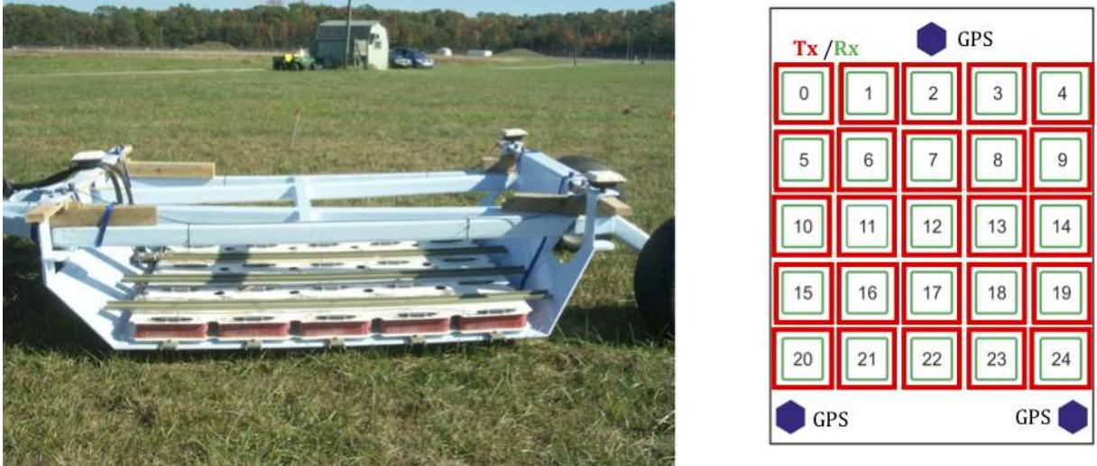
Figure 3.6: Photo of the TEMTADS in deployment at Blossom Point Test Site (left) and a schematic diagram of its Tx/Rx sensors (right).
