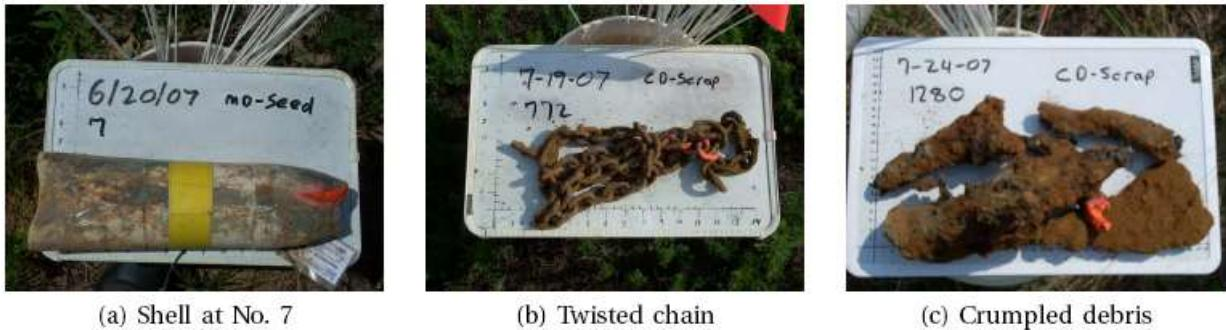
Figure 3.30: a) Unexploded shell from Cell No. 7 and (b,c) the two false alarms obtained by the SVM classifier using  $k$  and  $a$  as discriminators.
