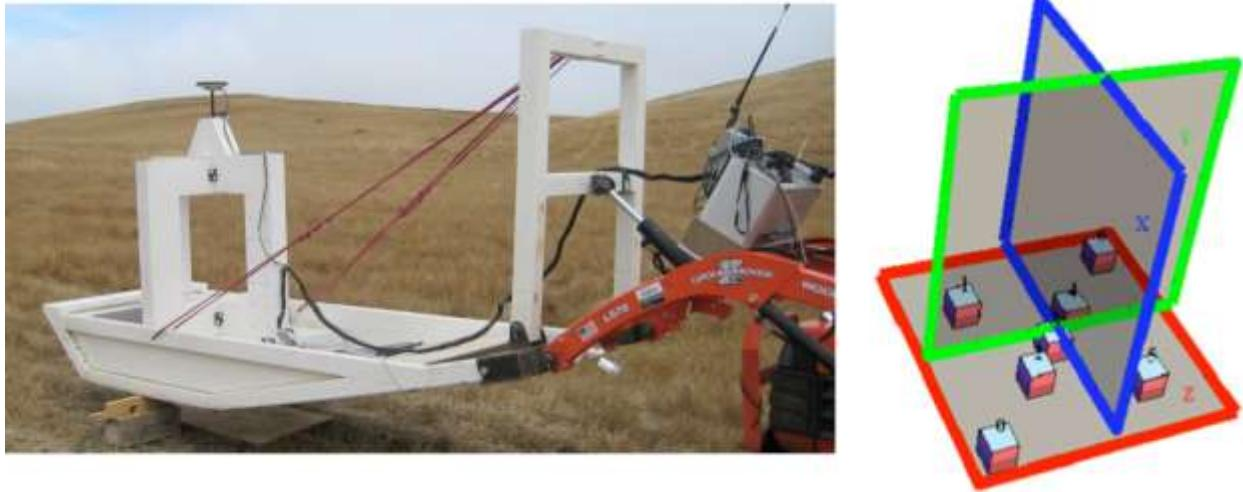
Figure 3.1: The MetalMapper during SLO site deployment (left) and its schematic diagram (right).
